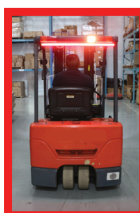
Forklift in reverse, rear light changes to RED
