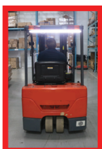
Forklift in drive, rear light remains WHITE
